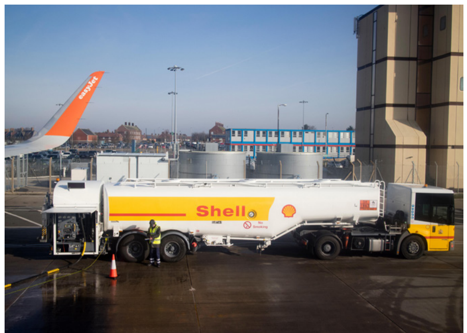
Shell oil jet-a1 refuelling tanker
